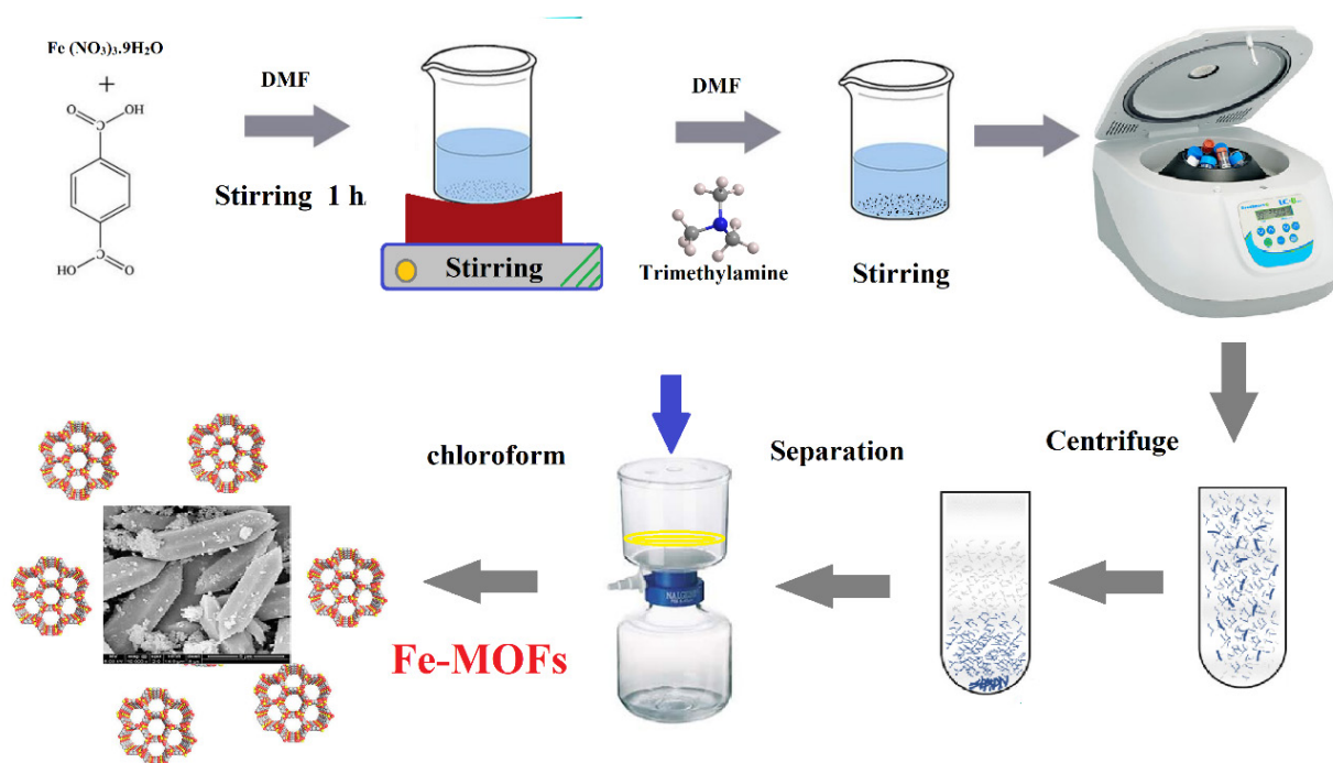
Schema 1. Preparation of Fe-MOFs by solvothermal method
